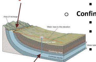
Well drilled into confined aquifer
