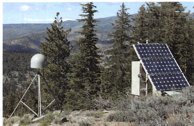
Figure 2.8 Example of a GPS station. Plate Boundary Observatory Station P150 on Martis Peak, California (lat 39.29238°, long -120.03386°). The antenna is under the gray dome to the left and is mounted on stainless steel pipes that extend ~15 m into the ground. Solar panels supply the energy for the electronics that acquire the data and transmit them elsewhere for analysis.
