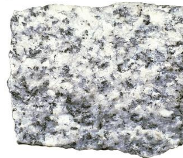
Platy and elongated mineral grains having random orientation.
