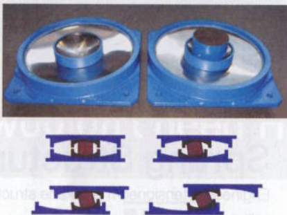
THREE-GEAR SLIDER Triple-pendulum bearing (top) is shown in upper and lower sections to reveal the three pendulums. Four cross-section sketches (above) show the isolator's static position (top left) and three positions during increasingly higher-magnitude earthquakes.
